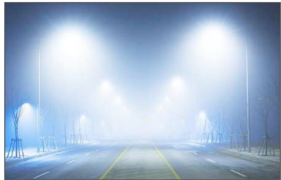
High glare with blue containing LED street lighting especially at foggy, snowy or winter conditions (3000- 6000K)
